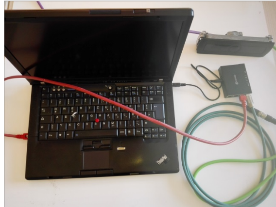
Fig. 6: Ethernet connection via ETH switch and via the RJ45 connector on the PC
