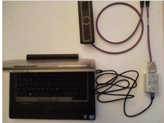
Fig. 8: CAN connection via the USB-CAN converter
